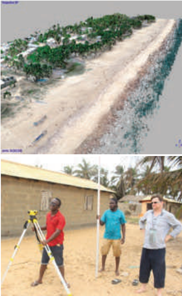
Oblique-angle photogrammetry-derived point cloud Topographic measurements with dumpy level
