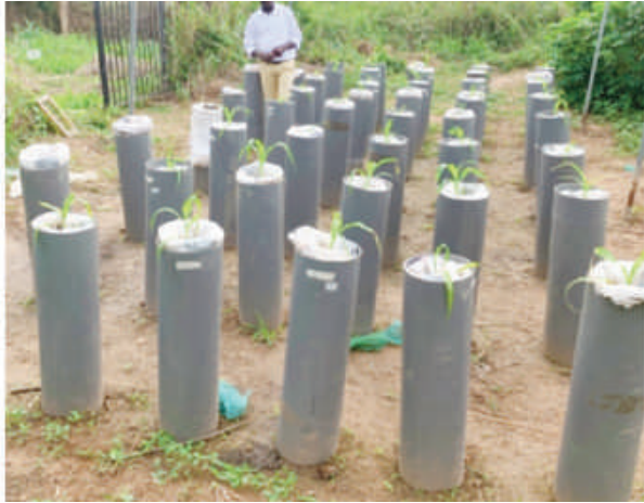
Sorghum plants growing in columns filled with soil at varying soil bulk densities and managed under varying soil moisture levels.
